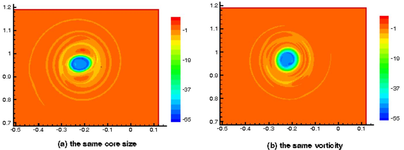
Figure 11. Vorticity contours after merging for the cases of co-rotating vortex merger in a two-vortex-pair system. (a) Same core size as in Fig. 9. (b) Same vorticity as in Fig. 10.
