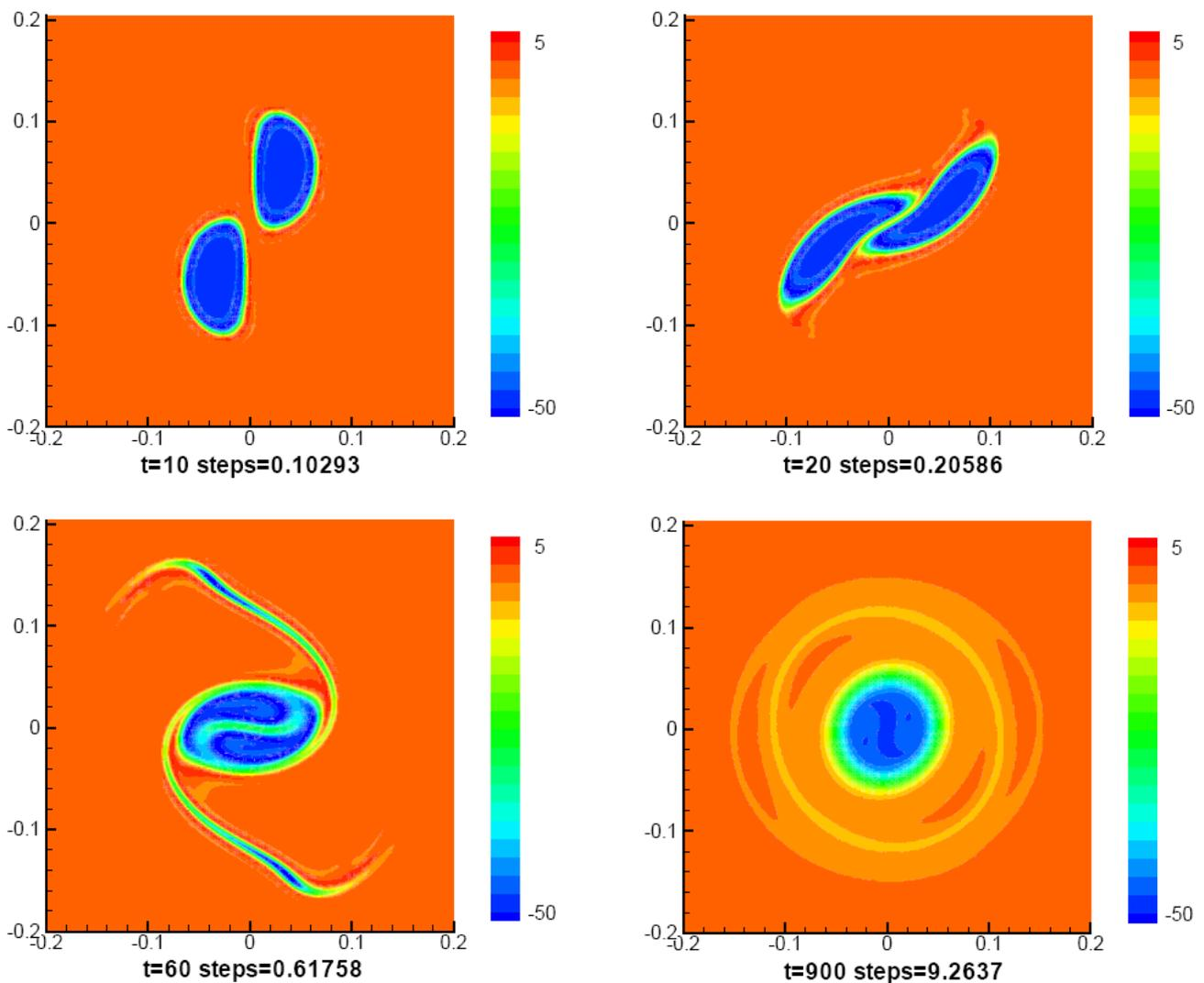
Figure 2. Snap shots of vorticity contours during the vortex merging process for the case with  $G = 0.126$ ,  $a = 0.042$ ,  $\beta = G/a = 3$ .
