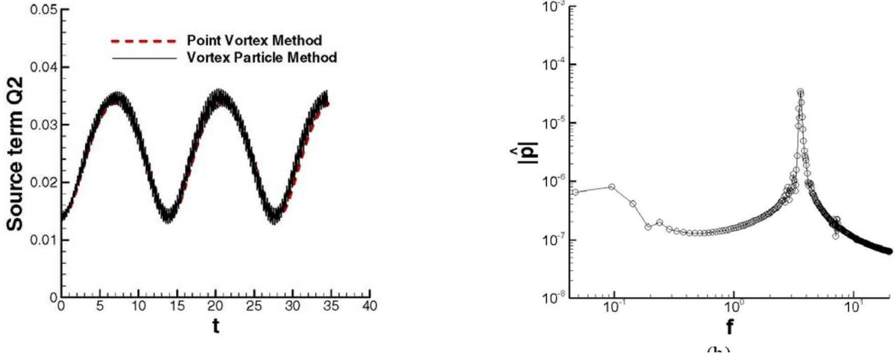
Figure 7. Two vortex pairs with the same vorticity and 1:2 ratio of the circulation without merging. (a) History of the quadrupole source term  $Q_2$  in Equation (12). (b) Spectrum of sound pressure magnitude in the frequency domain.
