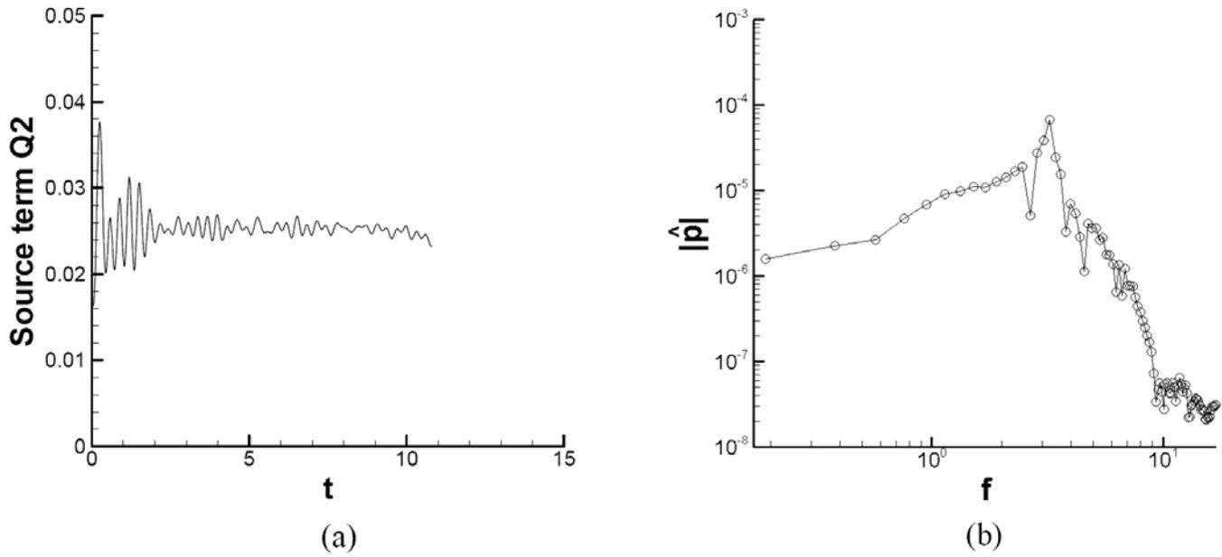
Figure 10. Two vortex pairs with the same vorticity and 1:2 ratio in circulation, with merging. (a) History of the quadrupole source term  $Q_2$  in Equation (12) (b) Spectrum of sound pressure magnitude in the frequency domain.
