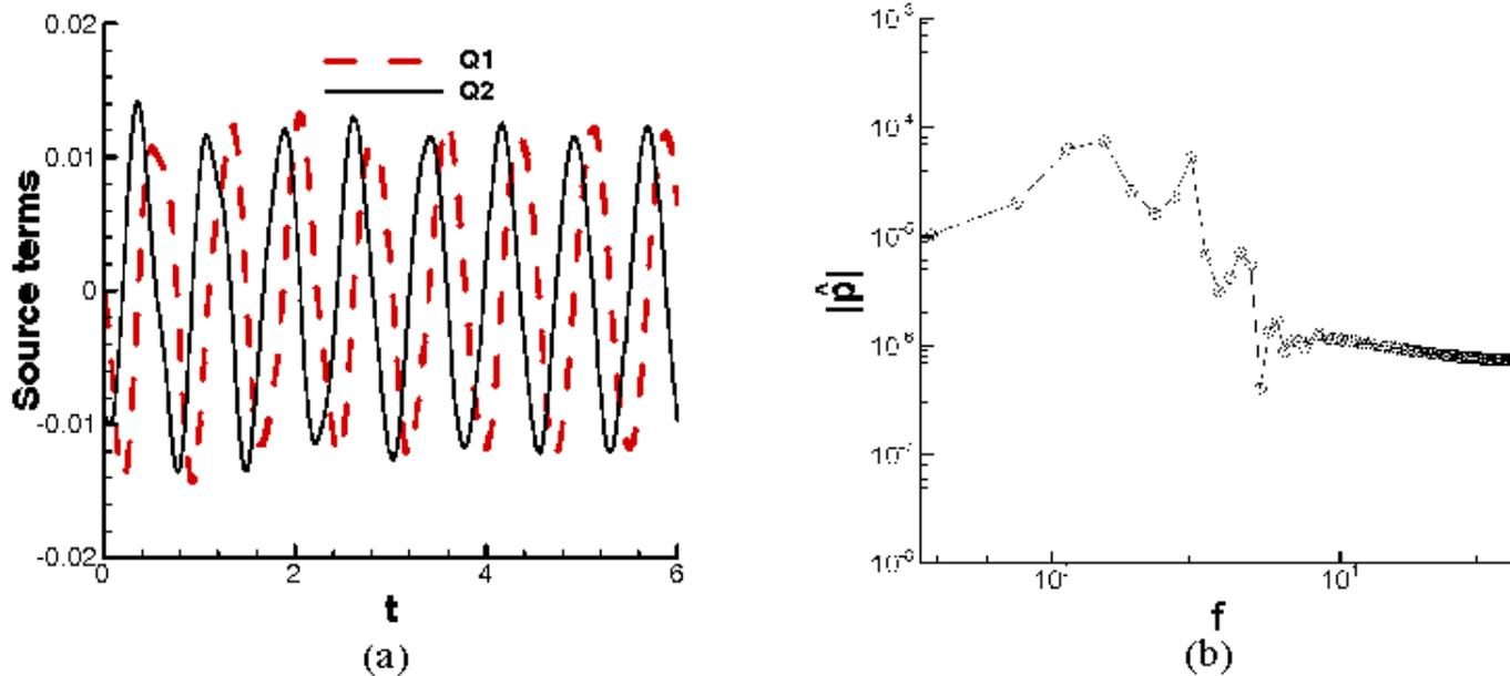
Figure 5. For the same case as in Fig. 4. (a) History of the quadrupole source terms in Equations (11) and (12) generated by two identical co-rotating vortices. (b) Spectrum of sound pressure magnitude in the frequency domain.
