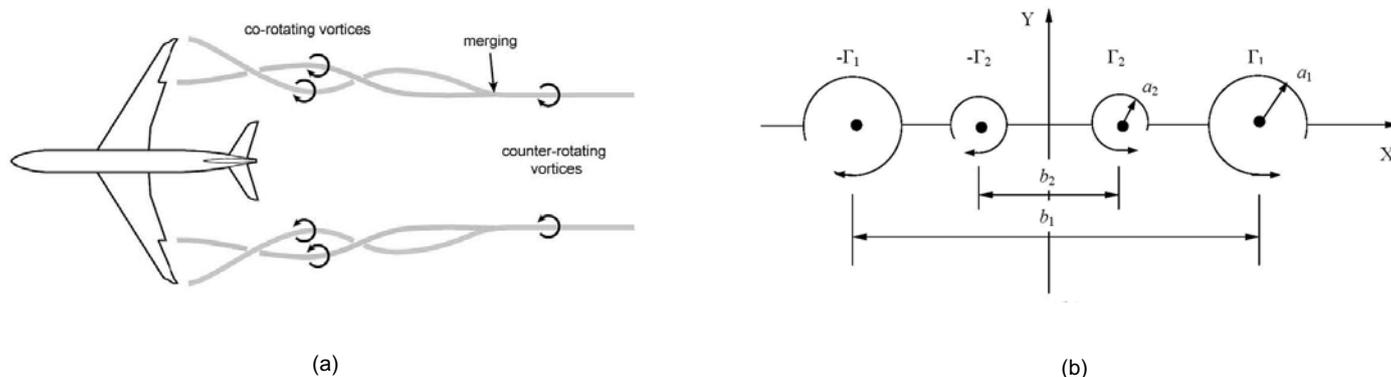
Figure 6. Illustration of (a) a typical aircraft vortex wake and (b) the initial setup of the multiple vortex pair system.
