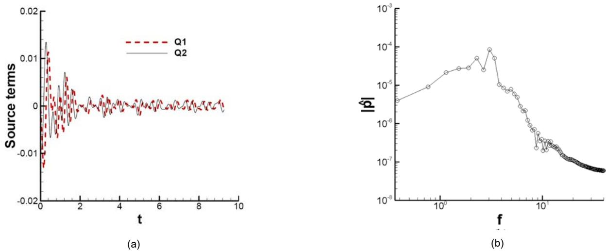
Figure 3. For the same case as in Fig. 2. (a) History of the quadrupole source terms in Equations (11) and (12) generated by two identical co-rotating vortices. (b) Spectrum of sound pressure magnitude in the frequency domain.
