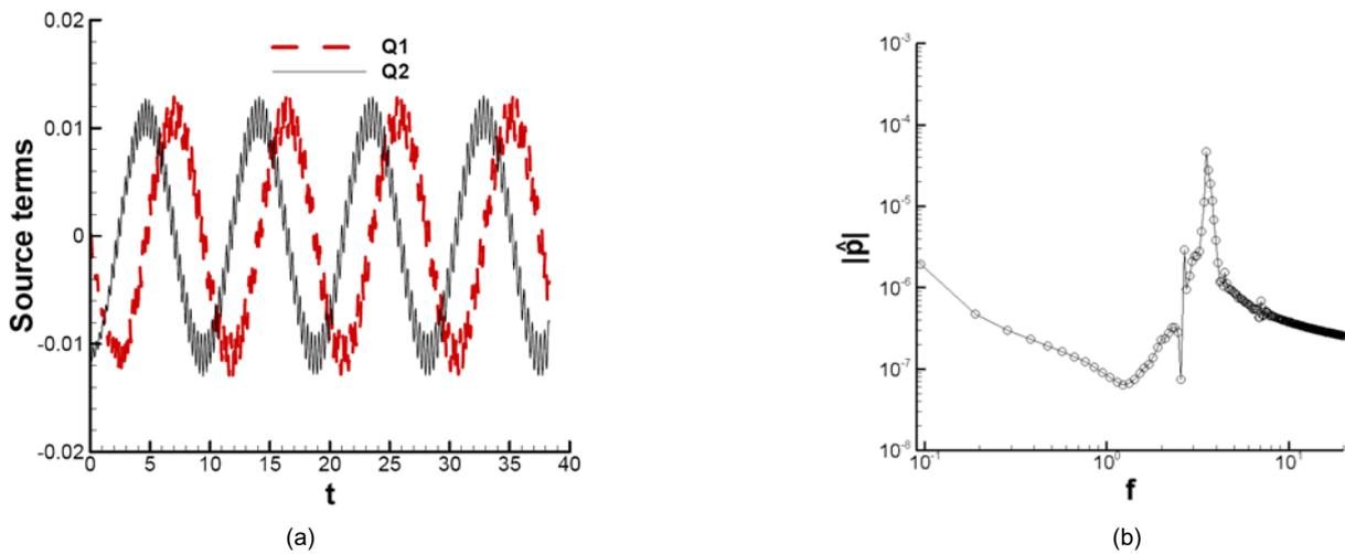
Figure 1. For the case with distance  $G = 0.5$ ,  $a = 0.042$ ,  $\beta = G/a = 11.9$ . (a) History of the quadrupole source terms in Equations (11) and (12) generated by two identical co-rotating vortices. (b) Spectrum of sound pressure magnitude in the frequency domain.
