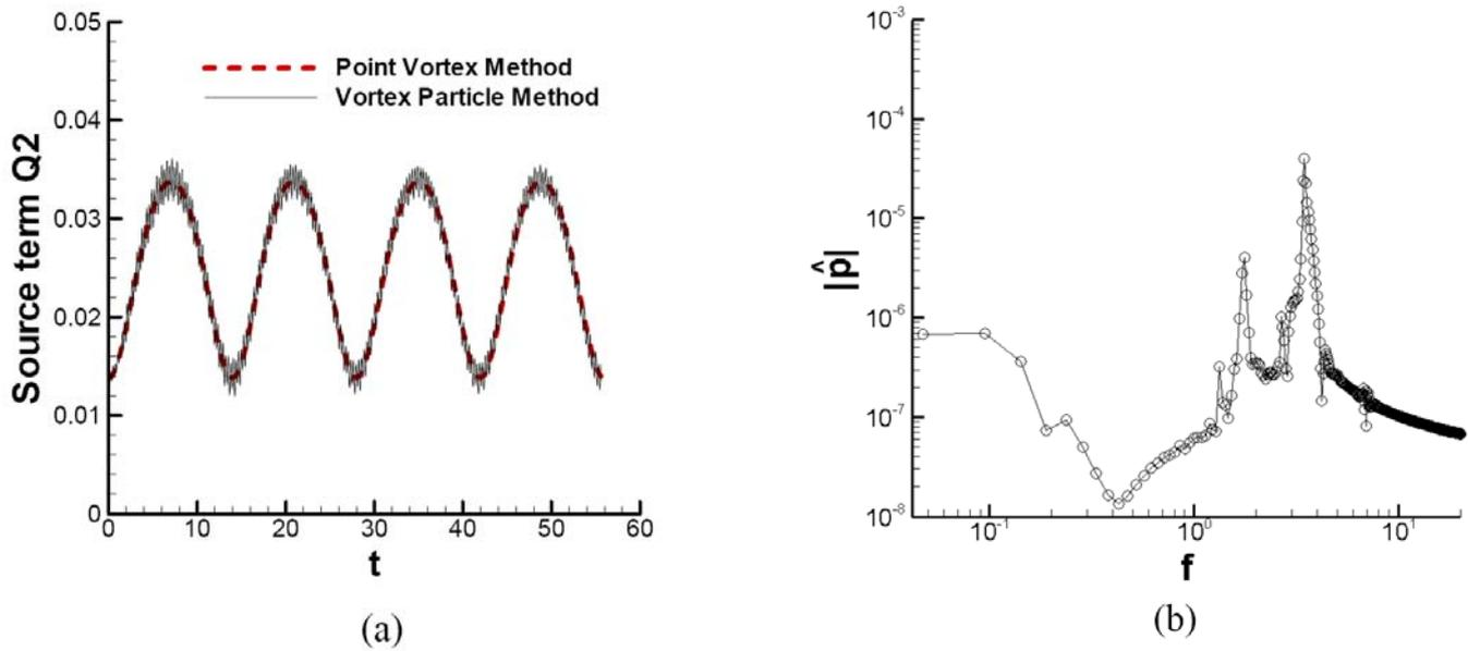
Figure 8. Two vortex pairs with 1:2 ratio in both the vorticity and circulation without merging. (a) History of the quadrupole source term  $Q_2$  in Equation (12). (b) Spectrum of sound pressure magnitude in the frequency domain.
