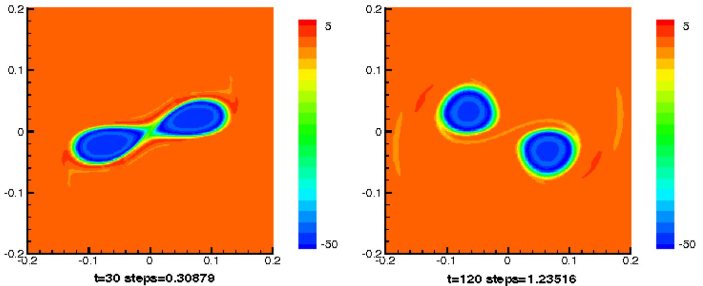
Figure 4. Snap shots of vorticity contours during the vortex merging process for the case with  $G = 0.147$ ,  $a = 0.042$ ,  $\beta = G/a = 3.5$ .
