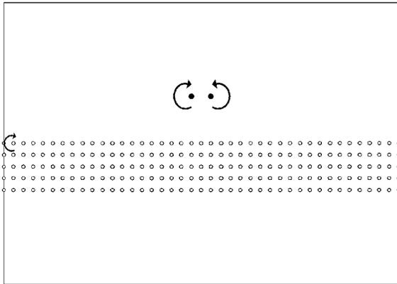
Fig. 1 Initial positions of vortices in the wake vortex/shear interaction model.
