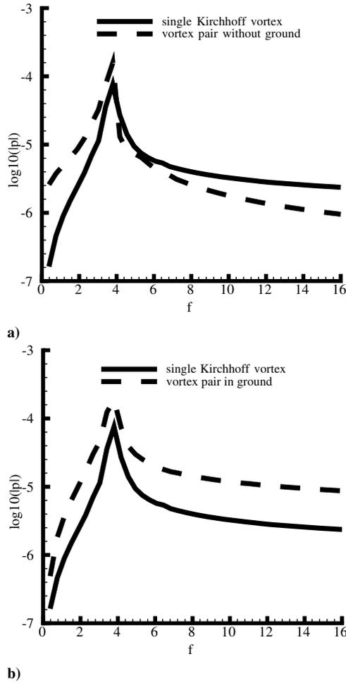
**Fig. 4** a) Comparison of simulated dimensionless spectrum of acoustic pressure between that of a single Kirchhoff vortex and that of a pair of counterrotating vortices; b) comparison of simulated dimensionless spectrum of acoustic pressure between that of a single Kirchhoff vortex and that of a pair of counter-rotating vortices with the ground image.
