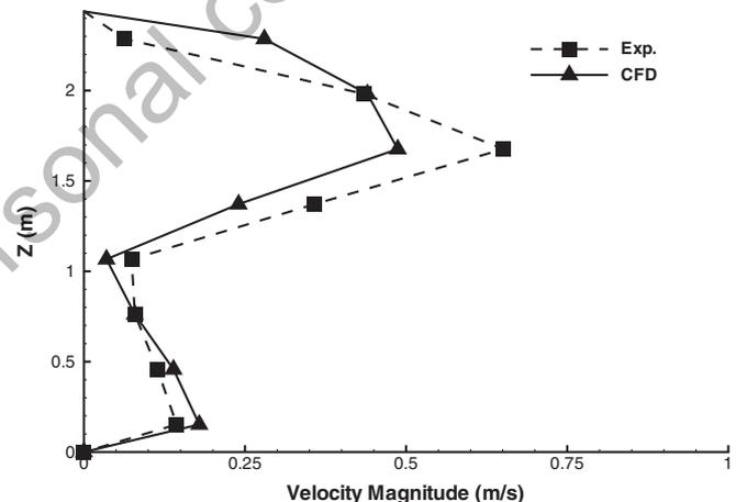
Fig. 3: Variation of velocity magnitude with vertical locations at the center of the chamber.
