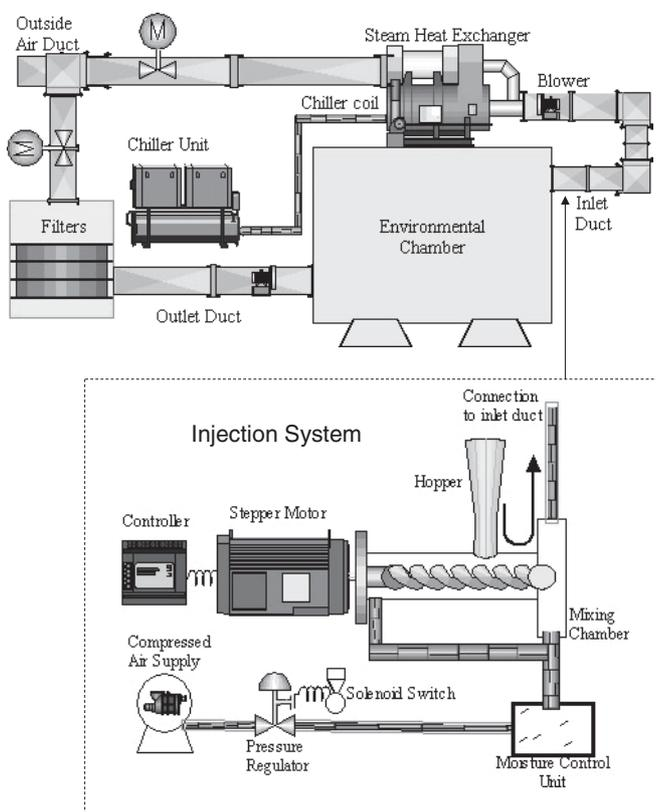
Fig. 2: Illustration of experiment system and particle injection system setups.
