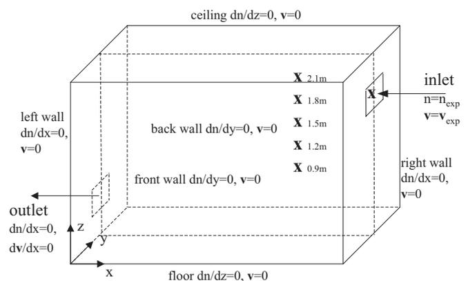
Fig. 1: Illustration of the test chamber, coordinate system and the boundary conditions. Symbol “x” represents the measurement locations.
